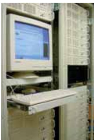
The new Linux cluster mill with 66 CPUs.
