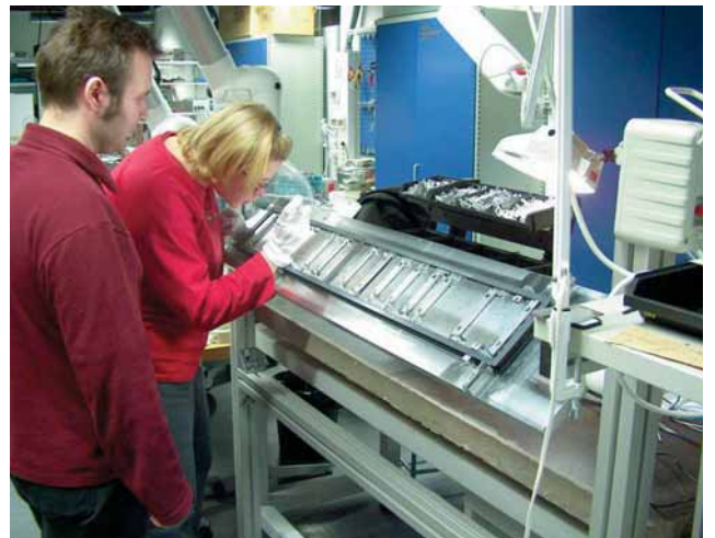
Support structure for the CMS Tracker Outer Barrel silicon detector modules being assembled at the Kumpula Laboratories.
