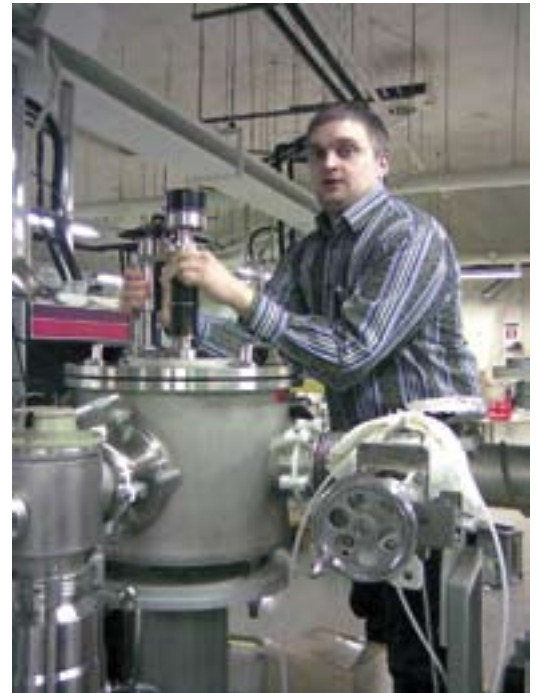
Samuli Väyrynen installing our silicon detector for irradiations at the HU Accelerator Laboratory.
