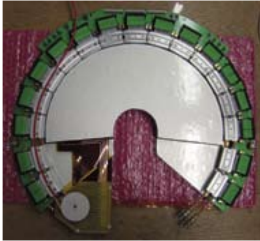
Final construction of a single TOTEM T2 GEM detector.
