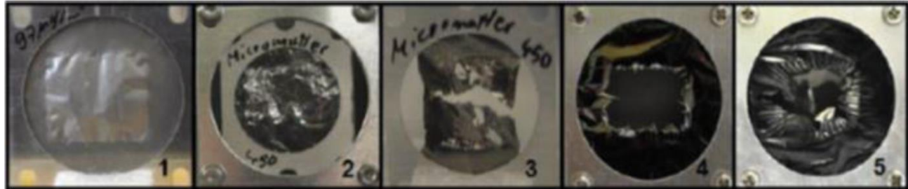
Different carbon foils irradiated with different ions to the same fluence, but pulsed and quasi-continuum beams, comparison made at FAIR/GSI.
