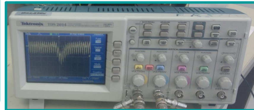
Noise of 32 MHz from Explode clock in the trigger lines
