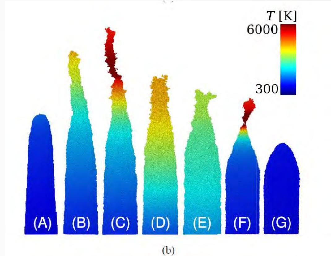
**Figure 5.** (a) Evolution of the height of the tip (red line, left axis) and the Cu atoms evaporation rate (blue dashed line, right axis). The designated points ((a)–(g)) correspond to the frames depicted in figure (b). The color coding of (b) corresponds to the local temperature. All evaporated atoms and nano-clusters have been removed. The full animation is available in the supplementary material.
