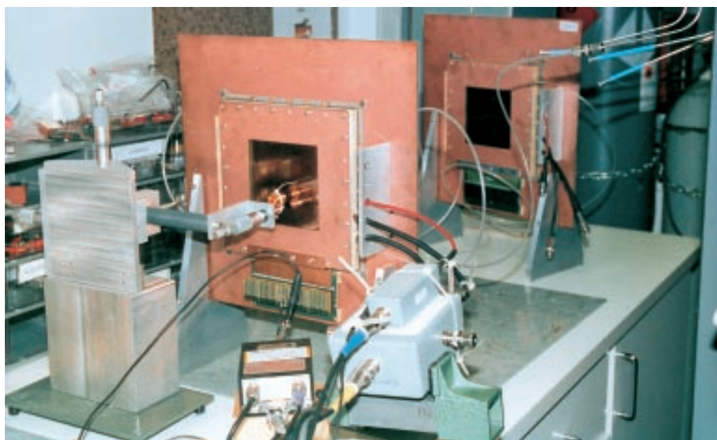
Fig. 4. The GEM detectors (manufactured in collaboration with CERN) under operational testing in the Innopoli detector laboratory of HIP.
