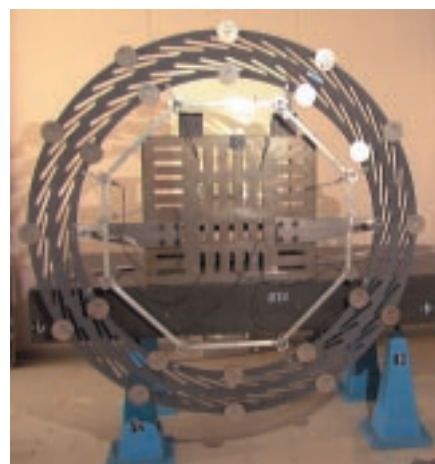
Fig. 1. The design and the manufacturing method of the MSGC support structure were verified by building first a smaller sector prototype and then a full-scale prototype of a two-layer disc supporting the two innermost layers of the final MSGC barrel. To measure the disc's static stiffness a water-cooled measuring frame equipped with capacitive probes was constructed.
