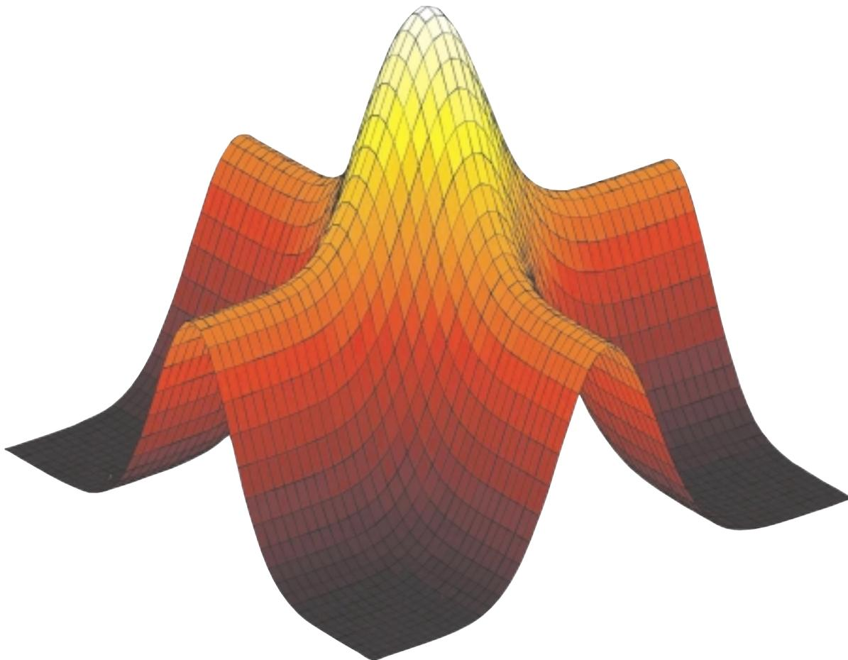
A sample trap for cold atoms and thus atomic Bose-Einstein condensates can be obtained by superimposing two laser beams which have Gaussian profiles. The atoms feel a force that pulls them to the localized field maximum. When an appropriate cooling mechanism is added, the atoms become trapped at that point.
