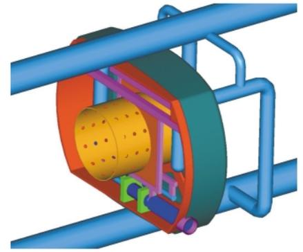
The inner architecture of a  $\mu$ station.
