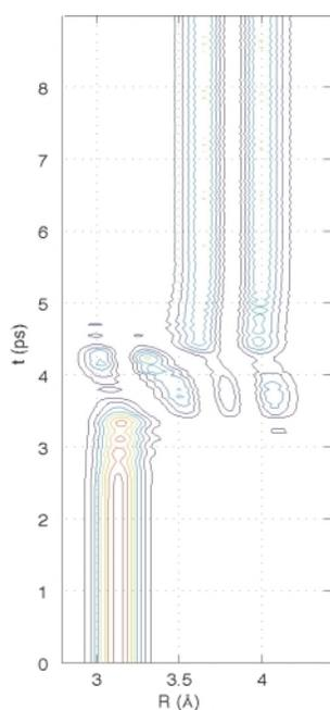
Using two short (in the picosecond range) laser pulses in counterintuitive order one can tailor the relative position of the atoms inside a sodium dimer molecule. The quantum mechanical position distributions are shown here as contour plots. The process induces strong quantum coherences between three electronic states, which result in selective change from one vibrational state to another.
