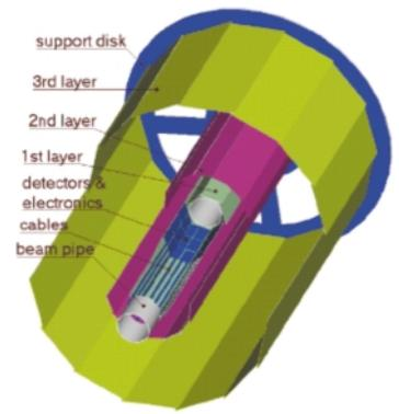
The design of a vertex tracker for a TESLA experiment.
