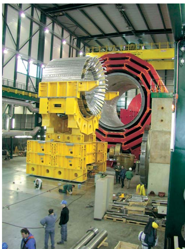
The CMS detector under construction in the surface hall of CMS. The large red rings form the return yoke of the magnetic field. The holes in the rings will host the muon detector units. The large steel cylinder inside the yoke is the outer wall of the vacuum tank of the superconducting solenoid that will create the magnetic field of 4 Tesla. The large cylindrical structure in the foreground is the hadron calorimeter that will be fitted in the space inside the magnet coil.
