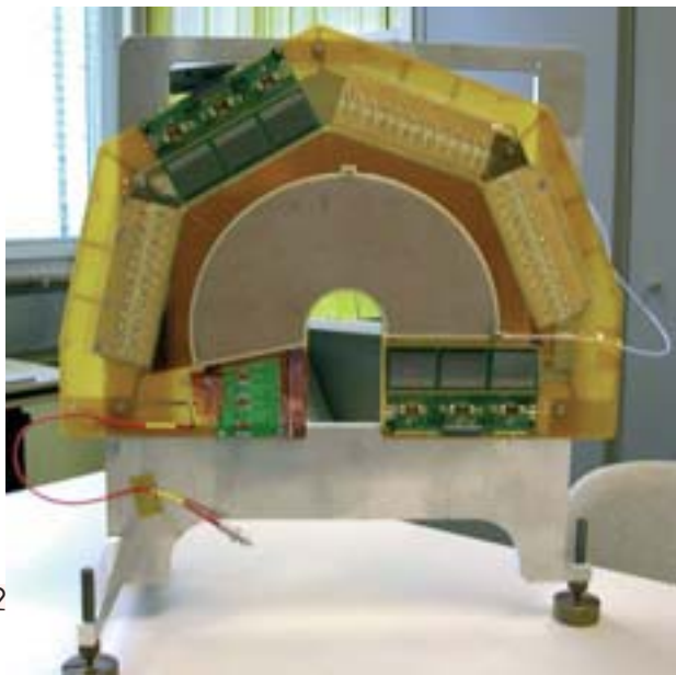
The first GEM prototype constructed for the TOTEM beam test in November 2004 at CERN.
