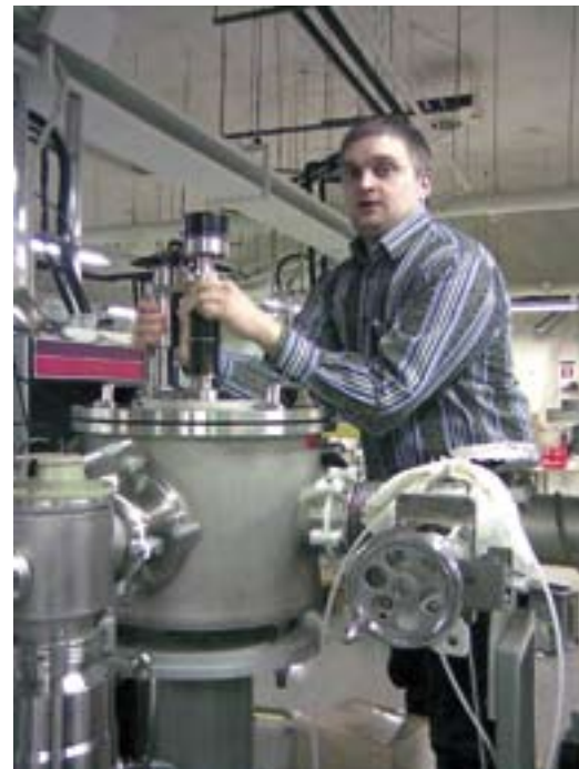
Samuli Väyrynen installing our silicon detector for irradiations at the HU Accelerator Laboratory.
