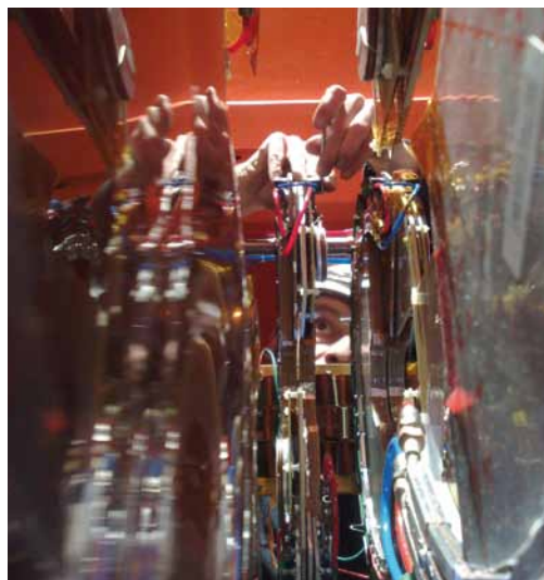
During the LHC winter stop in December three spare GEM detectors were replaced at the CERN T2 telescope.
