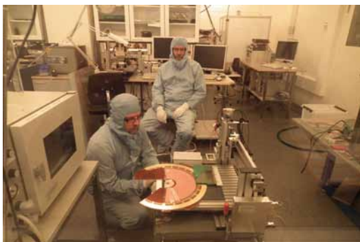
Totem T2 GEM structure being studied at the Detector Laboratory clean room.
