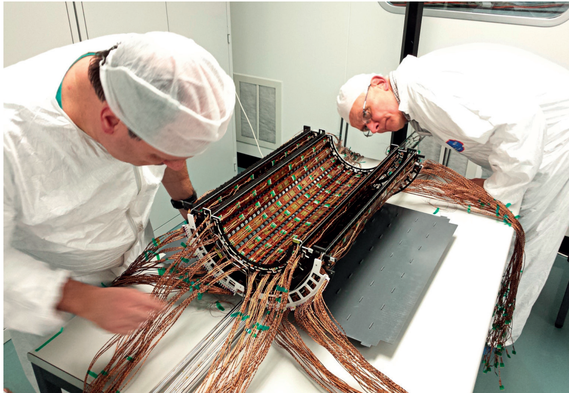
PSI researchers merging the CMS Barrel Pixel detector Layer 3 into Layer 4. The pixel modules produced in Finland are installed into Layer 3 and cover half of the whole layer. (Photo courtesy of R. Horisberger/PSI).
