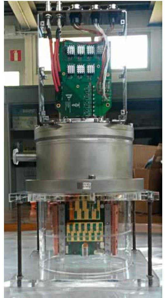
One of the CMS-TOTEM proton precision spectrometer diamond time-of-flight detector packages before installation in the LHC tunnel.
