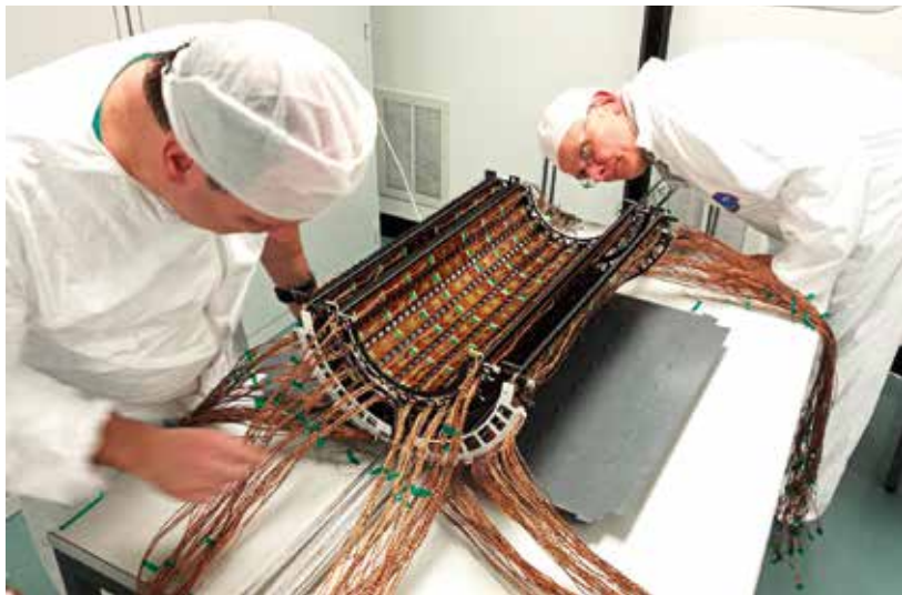
PSI researchers merging the CMS Barrel Pixel detector Layer 3 into Layer 4. The pixel modules produced in Finland are installed into Layer 3 and cover half of the whole layer. (Photo courtesy of R. Horisberger/PSI).
