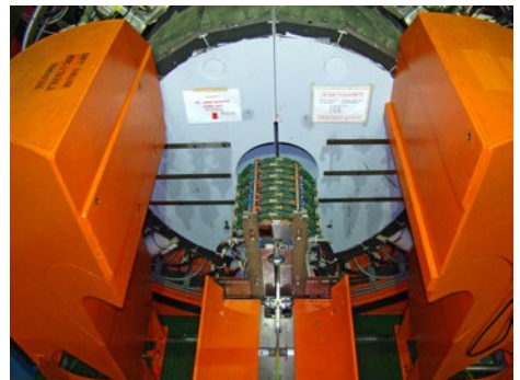
A fully commissioned T2 arm ready for insertion into the CMS hadron forward calorimeter (Photo: Jouni Heino).
