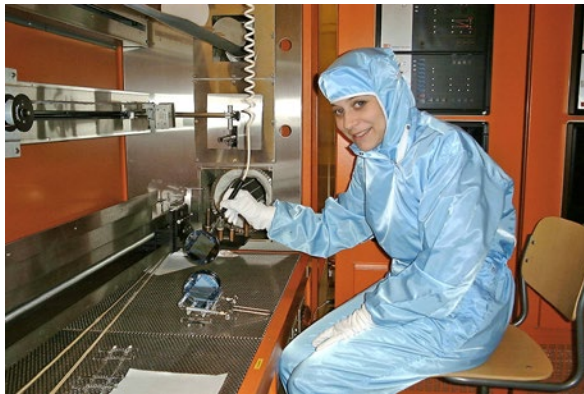
MSc Donatella Ungaro processing silicon strip detectors at the HUT Microelectronics Centre clean room (diffusion furnace).
