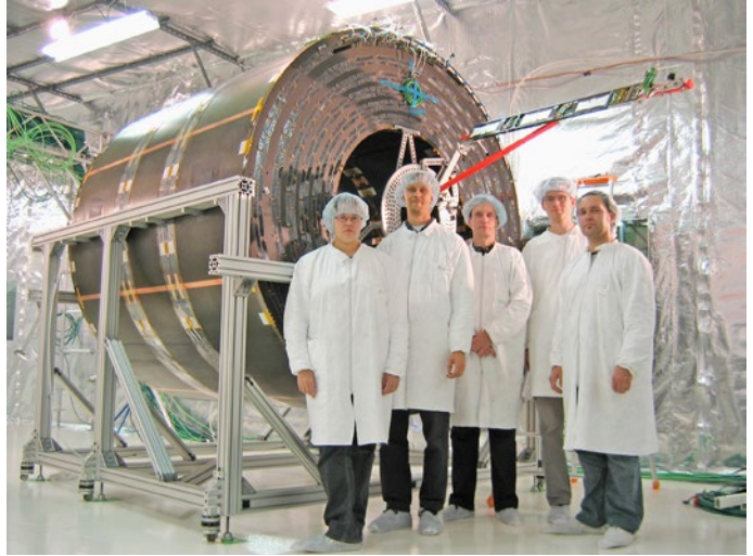
The HIP-CERN team, Auli Kuronen, Antti Onnela, Pauli Engström, Erkki Anttila, and Jarmo Korteesmaa, assembling the CMS Tracker Outer Barrel in 2005. At the top right, one can see one rod fixed to an assembly tool ready to be pushed into the TOB-Wheel (Photo: CERN).
