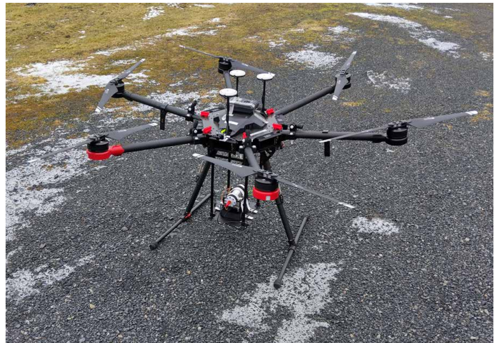
The Light-BISSE spectrometer being flown beneath a hexacopter in Jokioinen. Credit: M. Kalliokoski.
