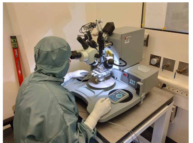
The first Single-point Tape Automated Bonding (SpTAB) attempts on the HIP cleanroom premises by P. Koponen. Credit: A. Nikkanen.
